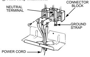
WARNING: THE NEUTRAL OR GROUND WIRE OF THE POWER CORD MUST BE CONNECTED TO THE NEUTRAL TERMINAL LOCATED IN THE CENTER OF THE CONNECTOR BLOCK. THE POWER LEADS MUST BE CONNECTED TO THE OUTSIDE (BRASS COLORED) TERMINALS.
